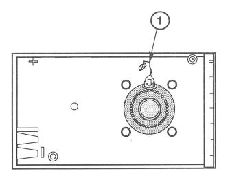
FIGURE 8 Speaker Wire Placement
