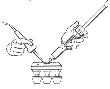
CAUTION: In the following steps, do not apply the soldering iron for more than three seconds. It may lift the traces off the board and destroy it.
