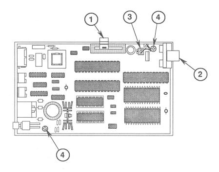
FIGURE 7 Main Logic Board and Speaker Removal
