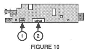
5. Slide the inner metal shield in the direction of the arrow in Figure 9 until the tabs on each side (Figure 10, #1) clear the holes; then lift off the shield. (If this is difficult, try carefully inserting a small flat-blade screwdriver under the shield to free it from the tabs.)
