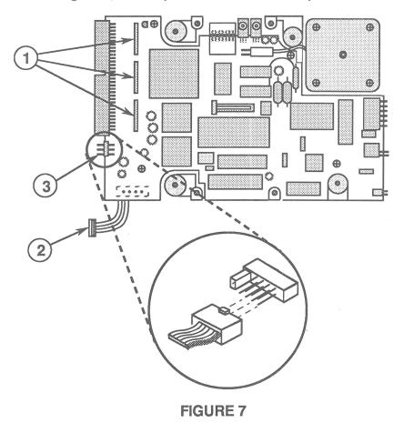
IMPORTANT: You must connect the customer's SCSI select cable to six unkeyed connector pins on the controller board. The SCSI connectors differ in design and location between drive models. For models represented by Figure 7, be sure to install the SCSI cable with its tab ("key") pointing up. For models represented by Figure 8, be sure to install the SCSI cable with its tab pointing toward the outside edge of the controller board.
